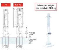
For fixation on finished floor Monclac floor standing bracket 120-215, article code R5209, the distance between the bottom of the radiator and the floor is adjustable per 5 mm.
