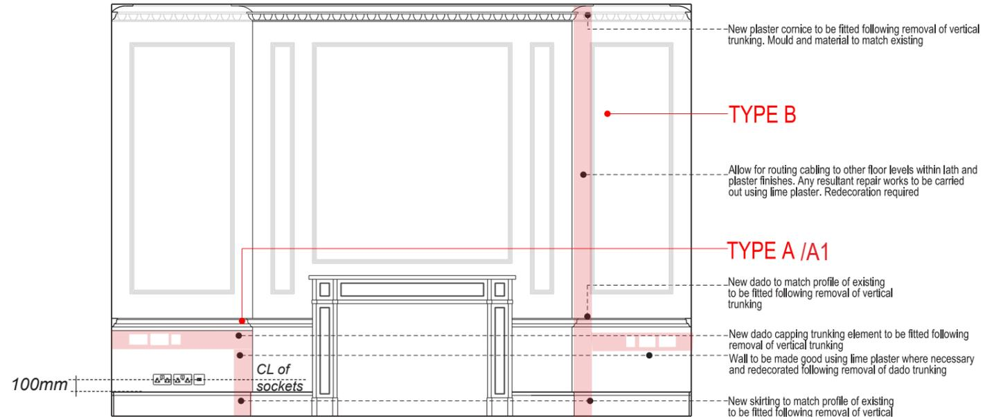
11MS/2/004 North Elevation - Additional Works Type A & Type B
