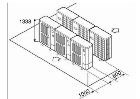
**NOTE:** CONTRACTOR TO SPECIFY AIR OUTLET GUIDE FOR CONDENSERS TO PROMOTE VERTICAL DISCHARGE & ACHIEVE CLEARANCES AS SHOWN
