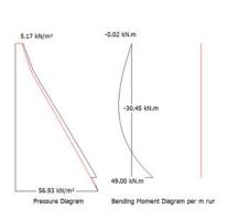
0.05 kN/m² Passive Pressure Diagram
