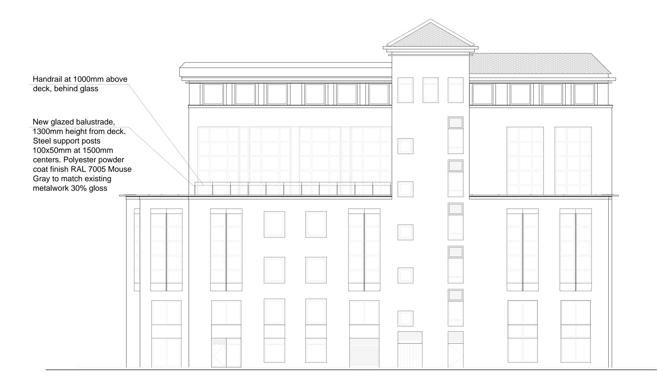
Notes: Do not scale from drawings. Contractor to site measure and verify all dimensions on site, and verify structural integrity. Refer to structural Engineer information for Structural design of balustrade.
