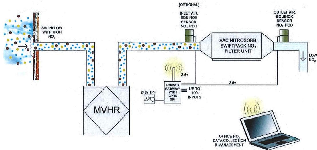
The schematic drawing above illustrates how EQUINOX® is positioned to provide end users with the critical information needed to measure the efficiency and performance of their installed AAC Swiftpack® NITROSORB® filter system.
