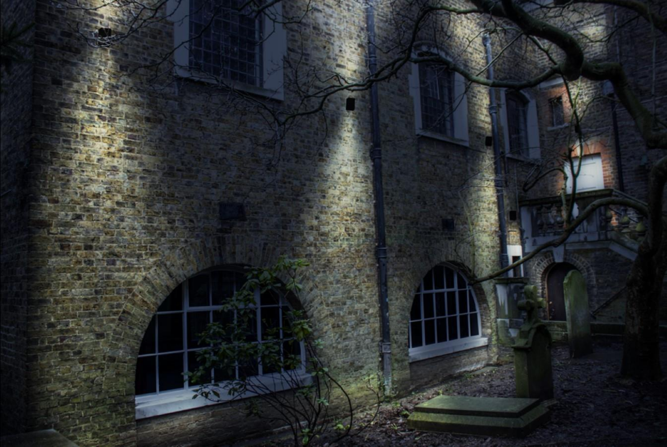
Up / downlight light to the building elevations and the pathway
