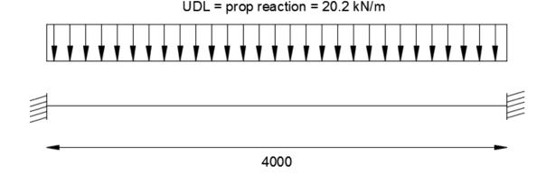
The actions on the rc beam therefore are:  $M= 1.6 \times w \times l^2 / 12 = 1.6 \times 20.2 \times 4^2 / 12 = 43.1 \text{ kNm}$  $S= 1.6 \times w \times l / 2 = 64.6 \text{ kN}$
