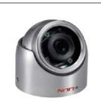
2Nos. cameras at the front door - Liliin IPC0422E4 covert camera finished in the same RAL colour of the existing wall. To be mounted within the door frame surround at high level. Each camera view will be fixed on the road and path directly opposite the property and will not have a PTZ (pan, tilt and zoom) feature. The camera dimensions are 130mm wide x 35mm high x 93mm deep.
