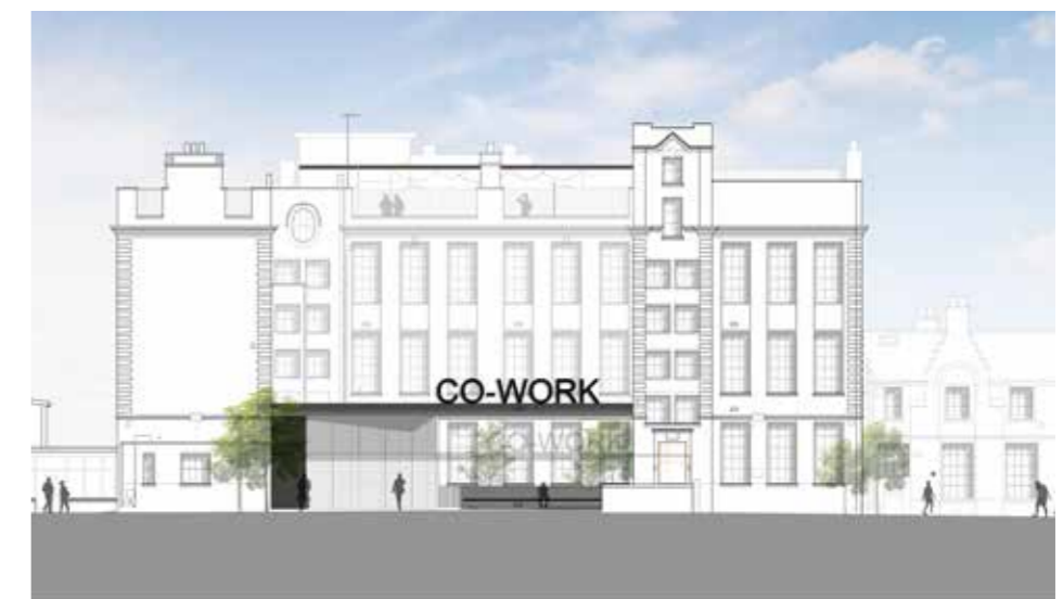
South Elevation with Proposed Entrance Pavilion
