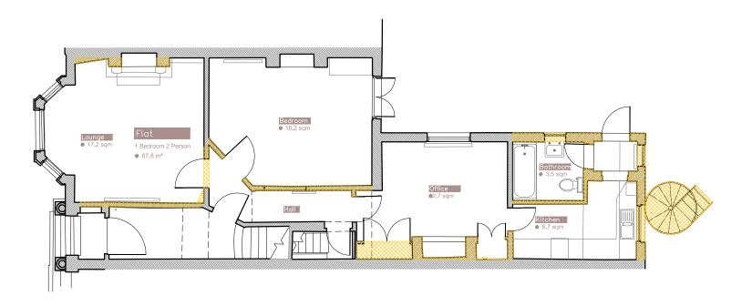
Demolition Ground Floor Plan - 1:100@A3
