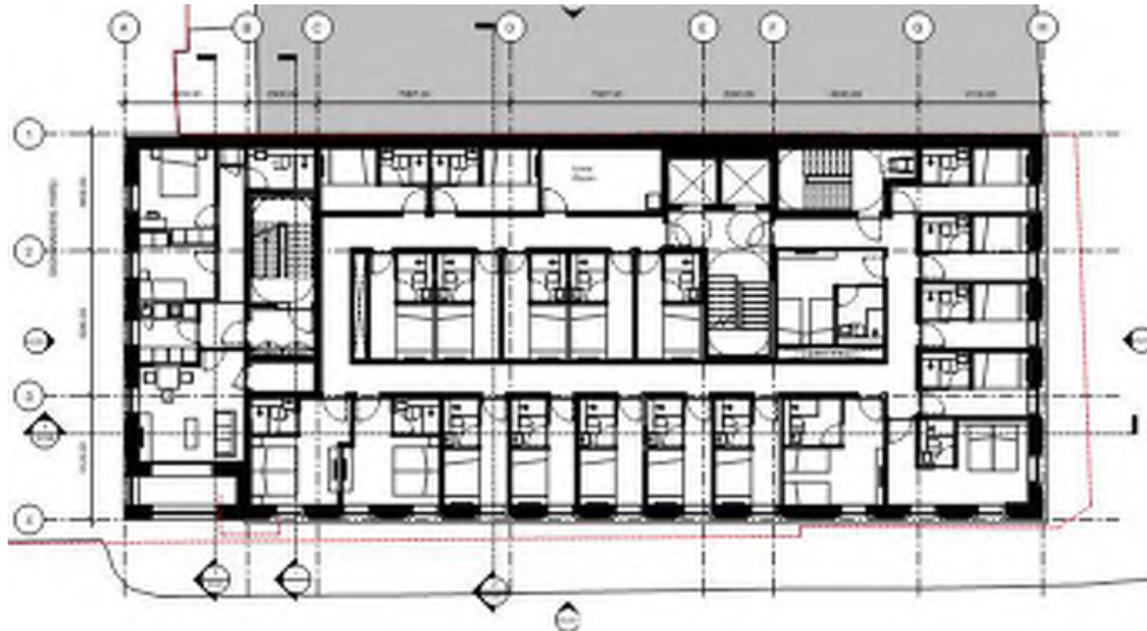
Figure 5 Proposed First Floor Plans (NTS)
