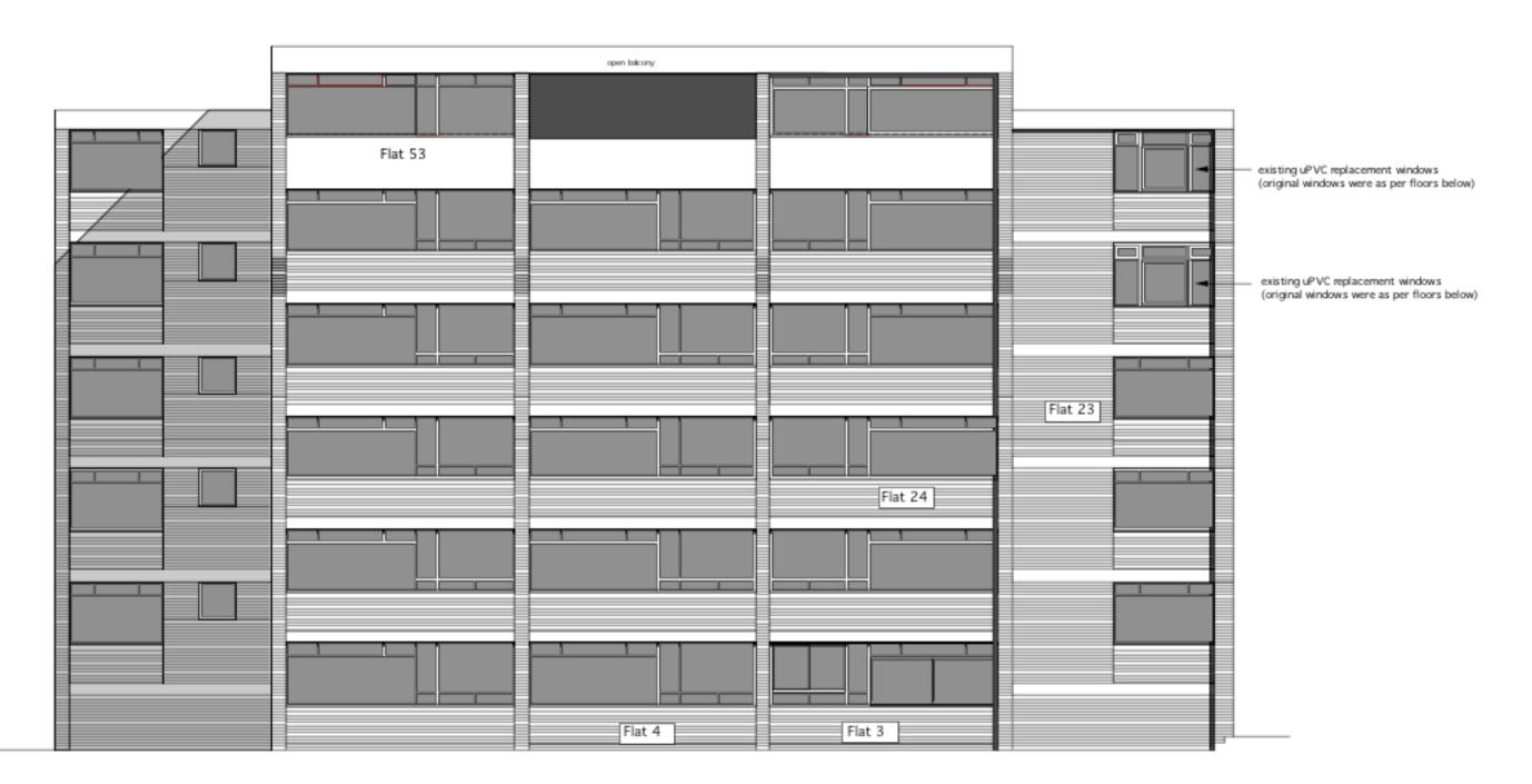
Existing Materials: Brick cross walls and brick panels between exposed floor concrete facias Concrete roof facias Concrete spandrel panels at 5th floor Tile hung spandrels ground to fourth Windows: brown painted hardwood single glazed
