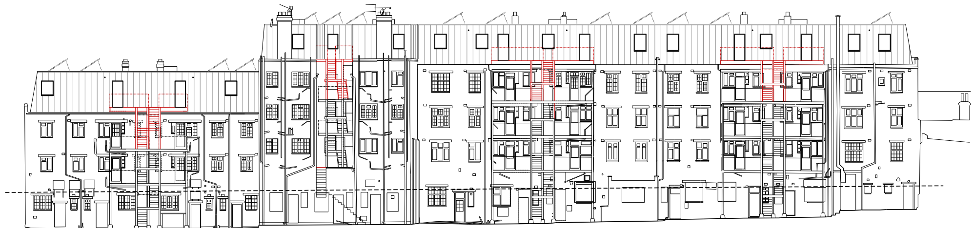
Proposed rear elevation, with the proposed extended external staircases shown in red
