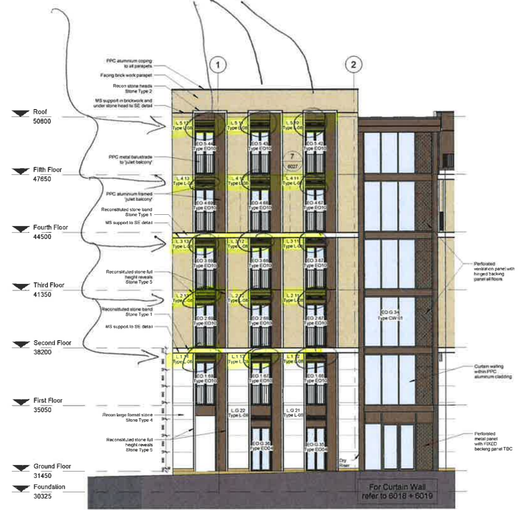
East Elevation (Southern End) 1 : 100
