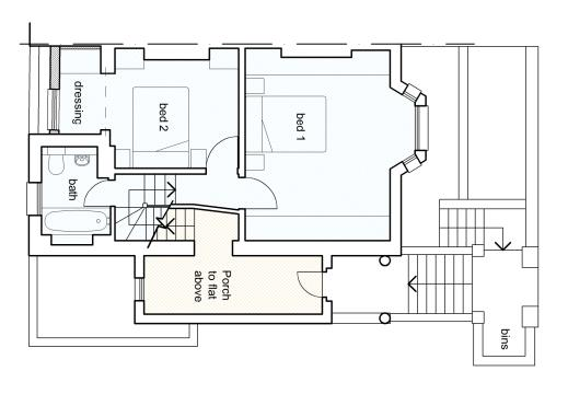
Proposed first floor plan Scale 1:100 @A3
