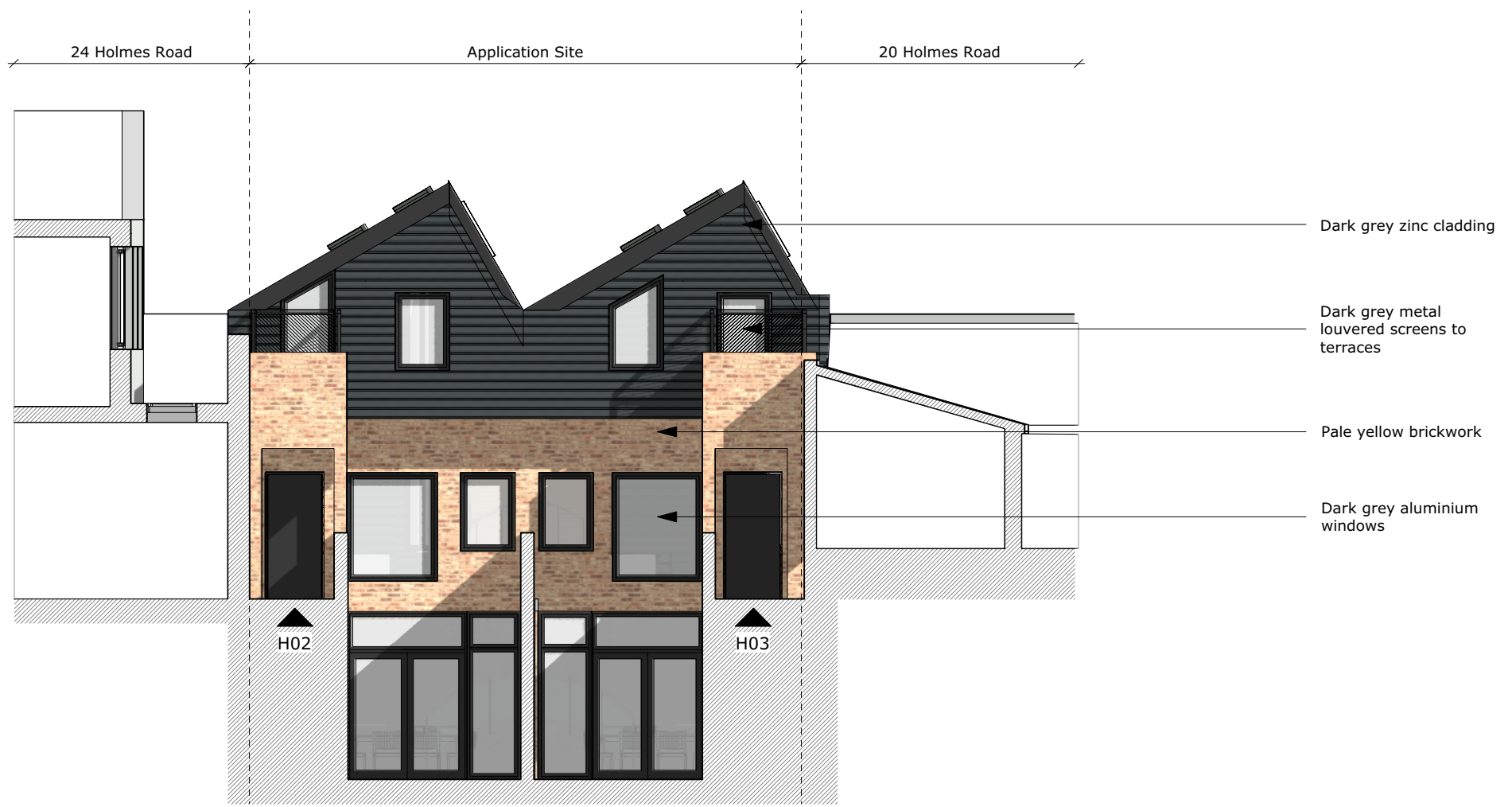
1 Courtyard Elevation H02 and H03 - Proposed Scale: 1:100
