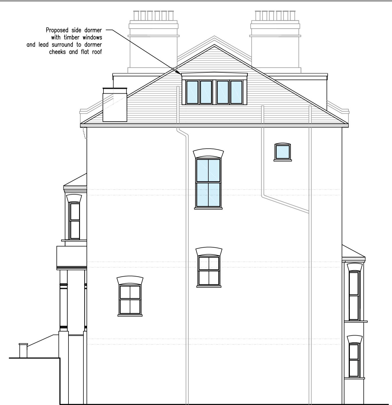
Proposed side elevation - Scale 1:100
