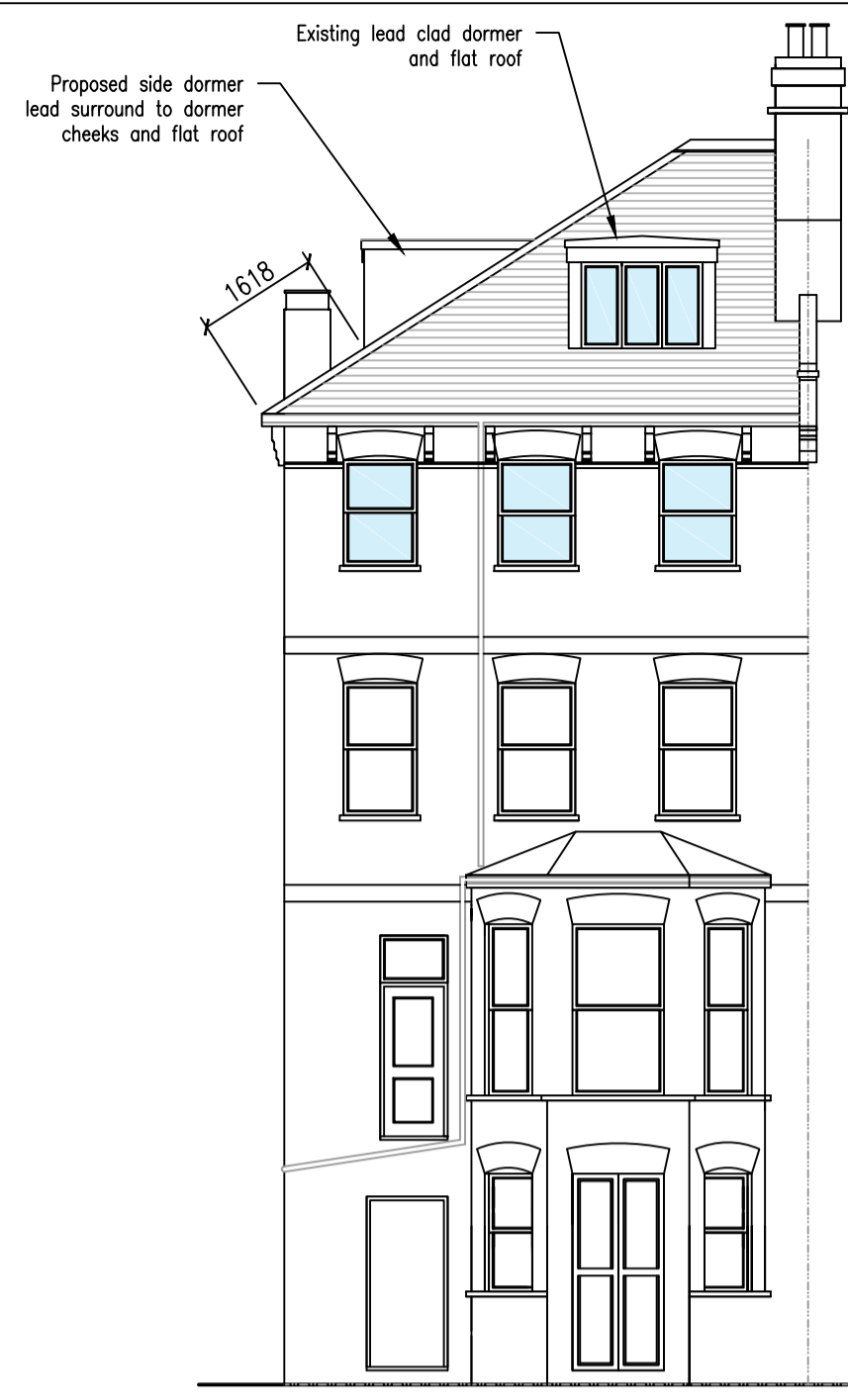
Proposed rear elevation - Scale 1:100
