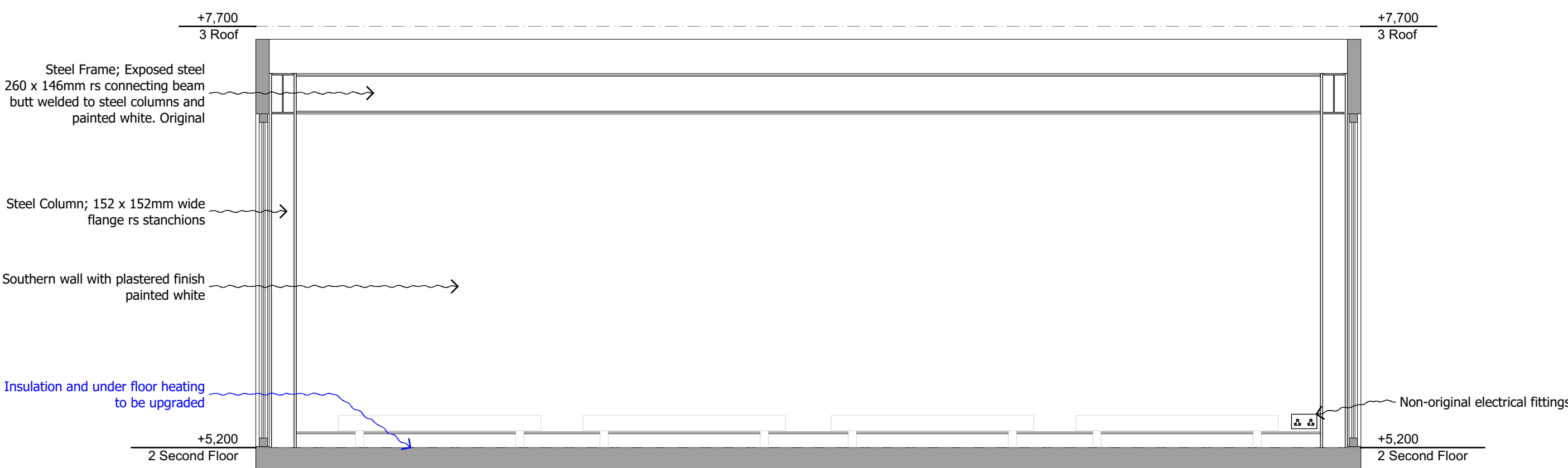
6 SCALE 1:25 @ A1, 1:50 @ A3 STUDY - ELEVATION 4
