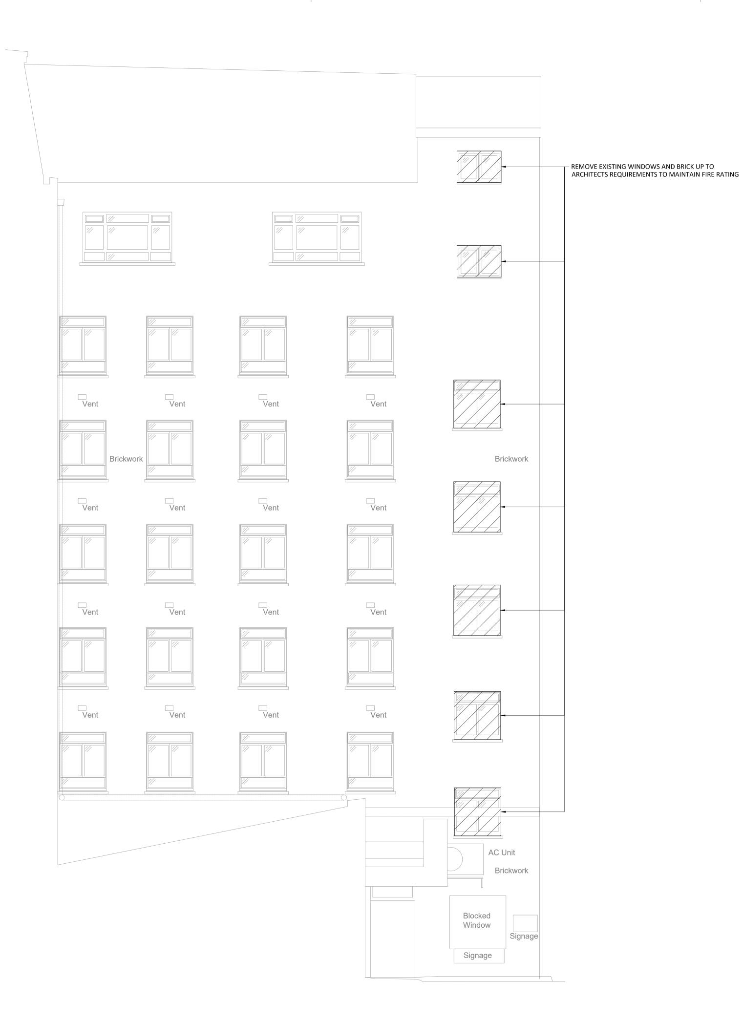
THIS DRAWING IS NOT TO BE USED FOR CONSTRUCTION. THIS DRAWING SHOWS DESIGN INTENT ONLY. THE CONTRACTOR SHALL COMPLETE THE DESIGN BASED ON THE INFORMATION PROVIDED ON THIS DRAWING, THE M&E SPECIFICATION, THE ROOM DATA SHEETS AND THE OTHER DOCUMENTS COMPILING THE EMPLOYER'S REQUIREMENTS
