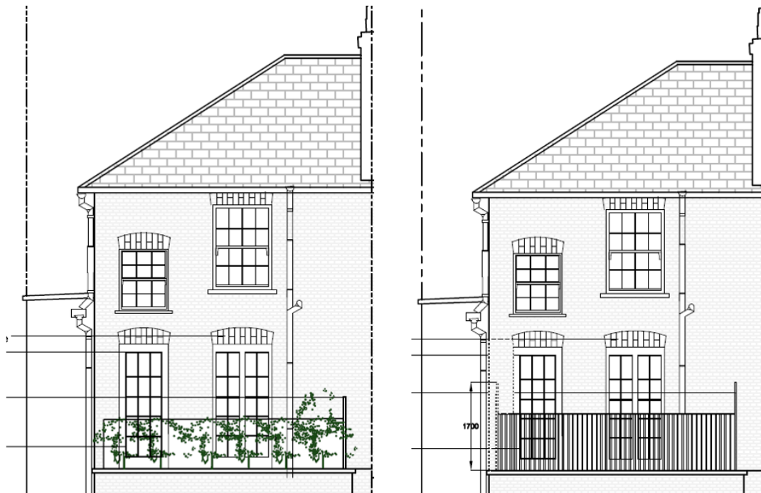
LEFT: PRE-APP DRAWING REAR ELEVATION RIGHT: FINALISED REAR ELEVATION WITH BLACK RAILINGS
