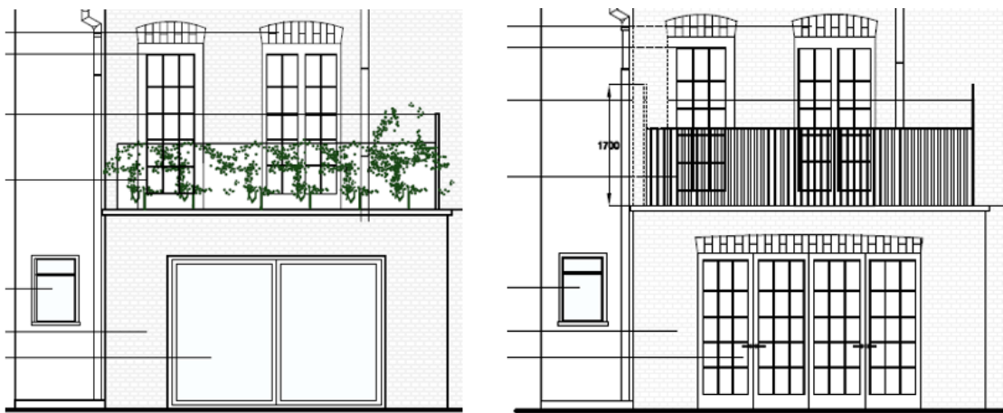
COMPARISON BETWEEN PRE-APP REAR ELEVATION (LEFT) AND AS REFUSED REAR ELEVATION (RIGHT)
