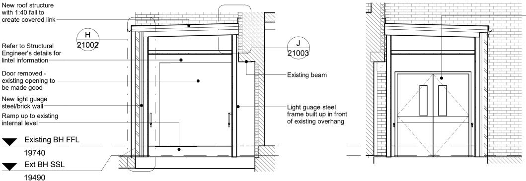
New doorset - existing opening to be widened to create required structural opening. - Refer to Door Types drawing 32010 and Door Schedule 06010
