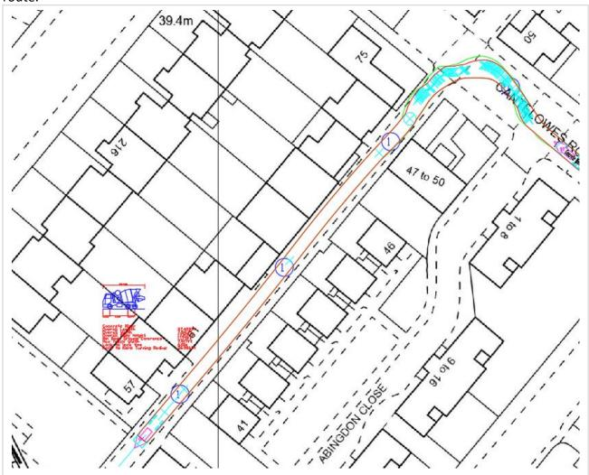
Swept path analysis above shows a concrete lorry which is predicted to be the largest vehicle to arrive at the site, turning from Cantelowes Road onto Camden Mews successfully.
