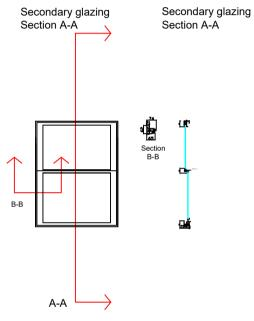
Existing single glazed timber window to be exactly same to keep the heritage look of the building and new secondary glazing to be fitted for thermal proposes to stop condensation and noises Notes:
