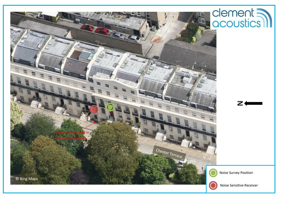
**14765-SP1** Indicative site plan indicating noise monitoring position and nearest noise sensitive receiver
