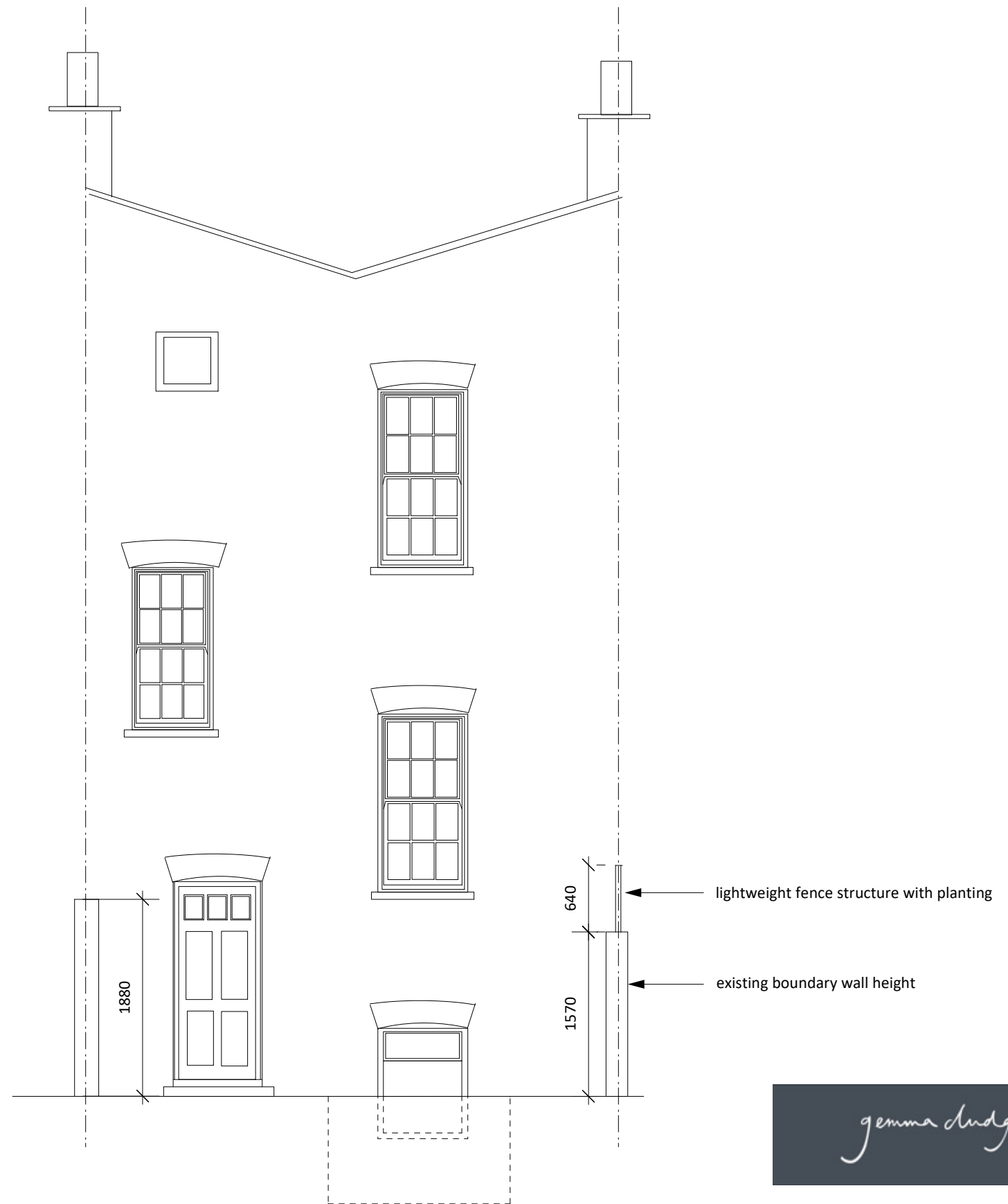
REAR ELEVATION AS EXISTING
