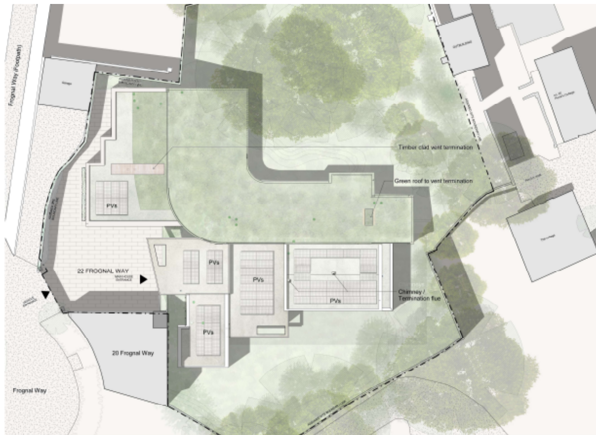
3) Proposed PV panel locations (on flat roof areas, not green roof); vents/chimneys/terminals also shown
