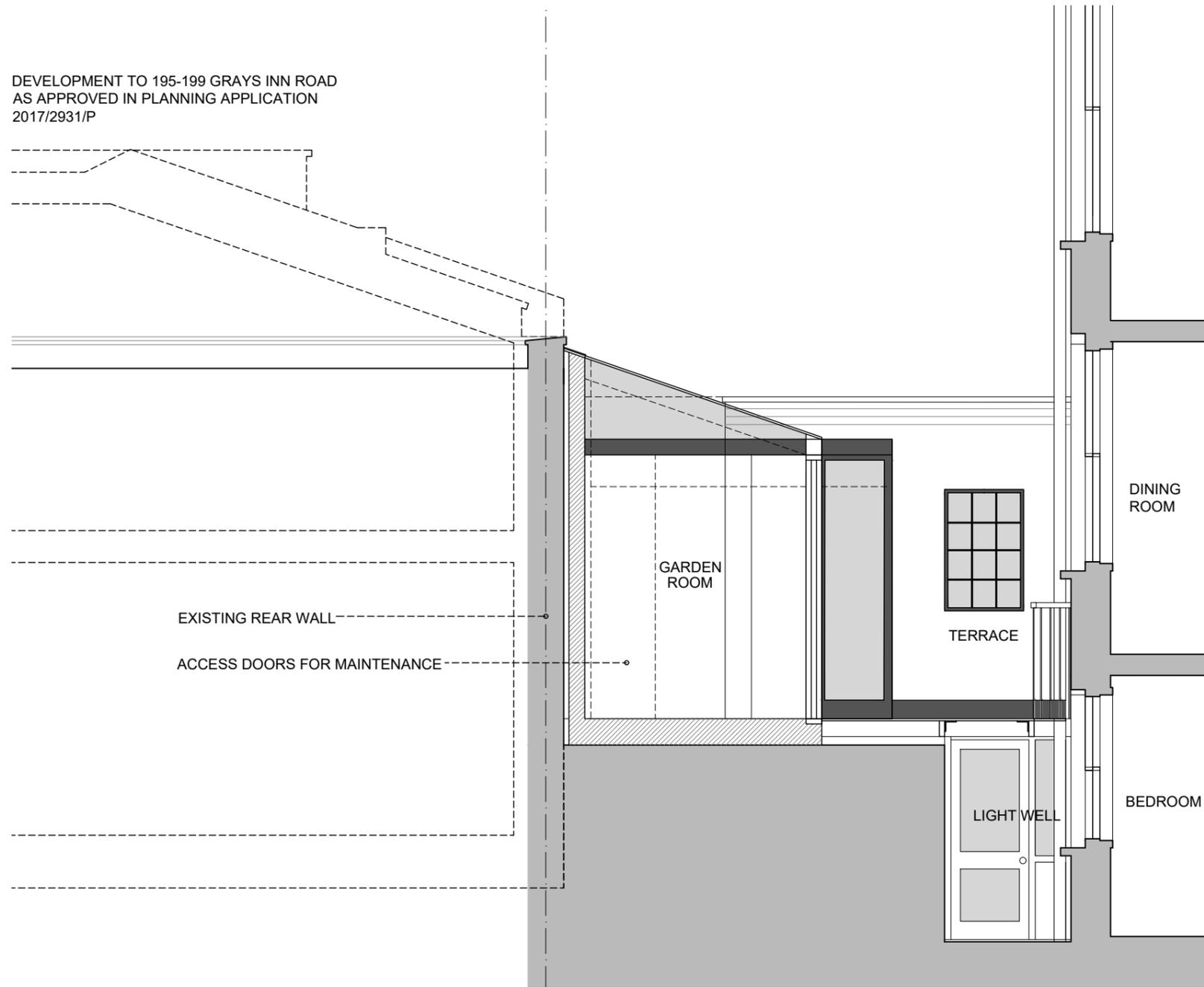
PROPOSED SECTION BB (INTERNAL ELEVATION)
