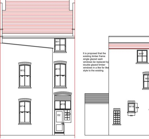
It is proposed that the existing timber frame single glazed sash windows be replaced by double glazed timber windows in a like for like style to the existing.
