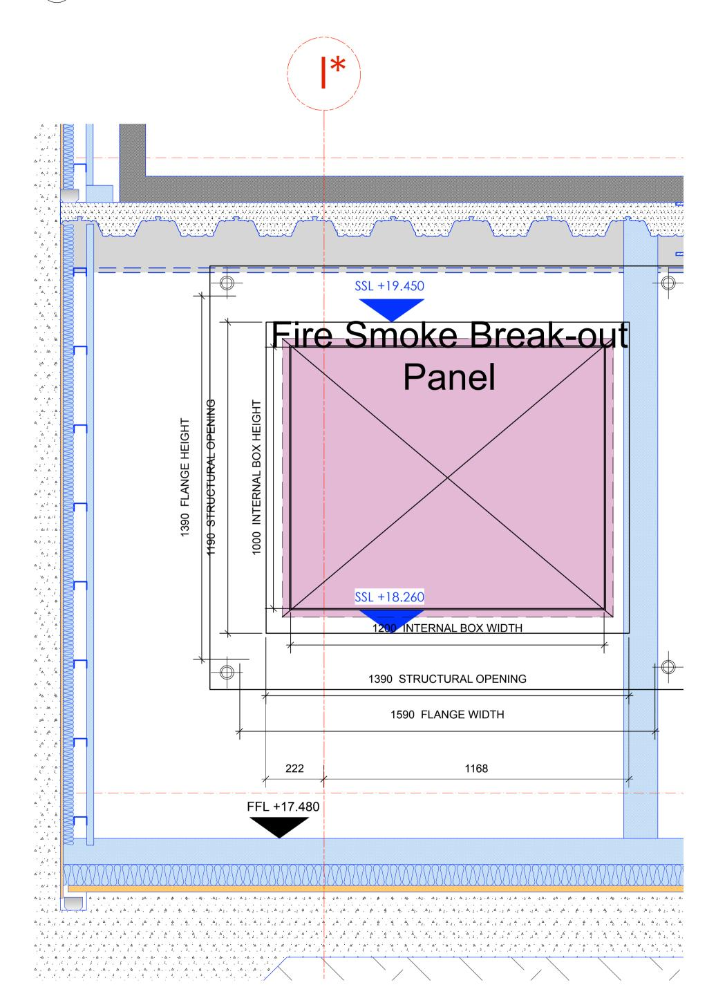
Inetrnal Elevation Opening size Scale: 1:10
