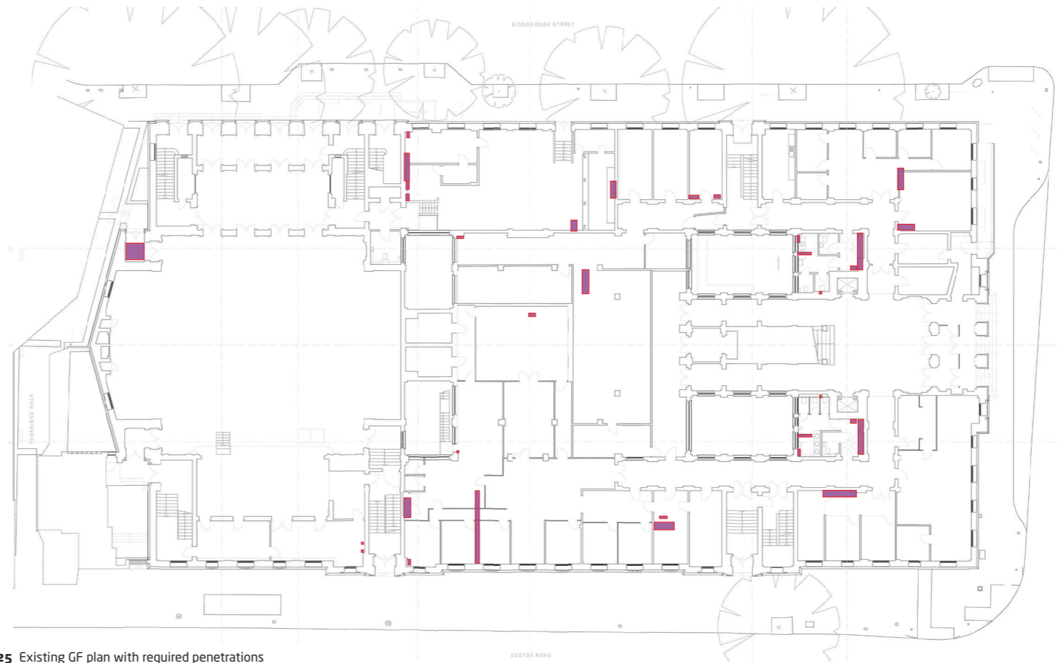
Figure 4.25 Existing GF plan with required penetrations
