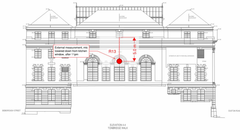
Figure 29: External measurement location, lowered down from the kitchen on Third Floor level of existing site
