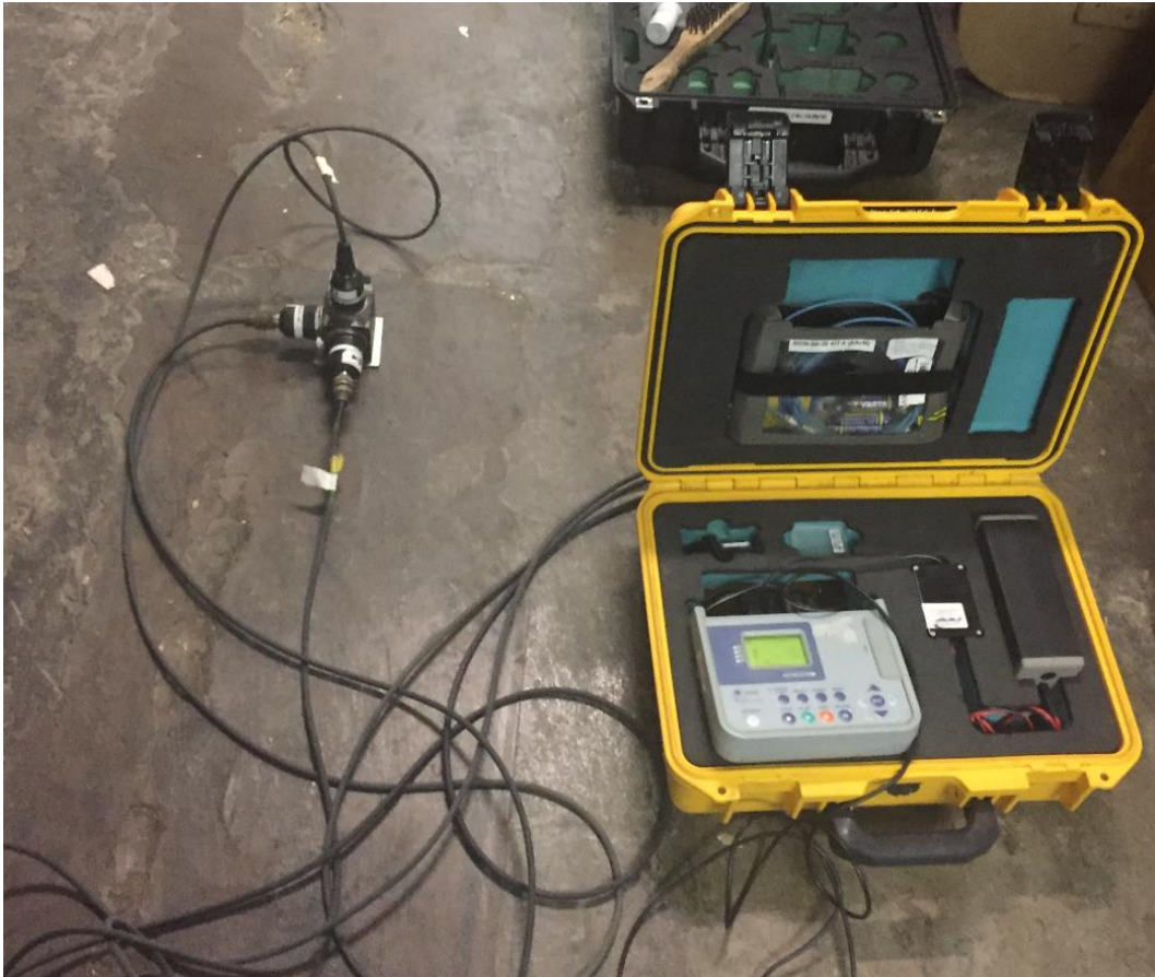
Figure 20: Set-up of vibration kit
