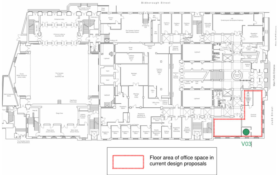
Figure 22: Vibration measurement locations at Ground Floor level in the existing building
