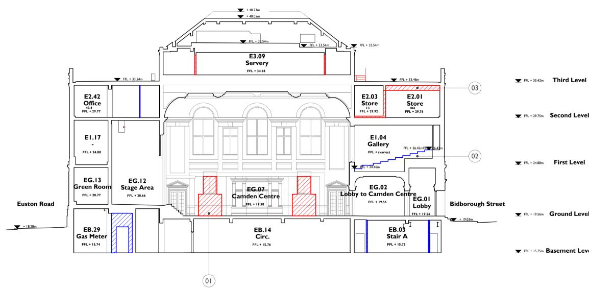
SECTION A-A PROPOSED DEMOLITIONS AND STRIP OUT 91200 I:200 @ AI
