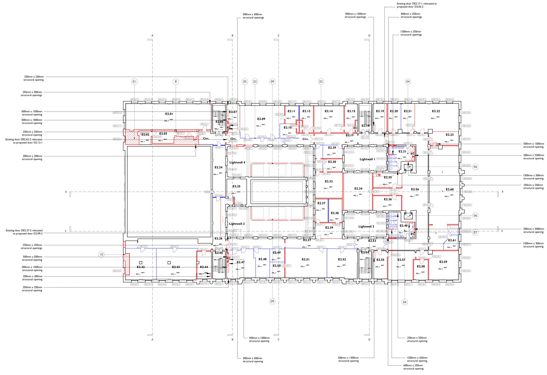
SECOND FLOOR LEVEL PLAN PROPOSED DEMOLITIONS AND STRIP OUT 91004 I:200 @ AI
