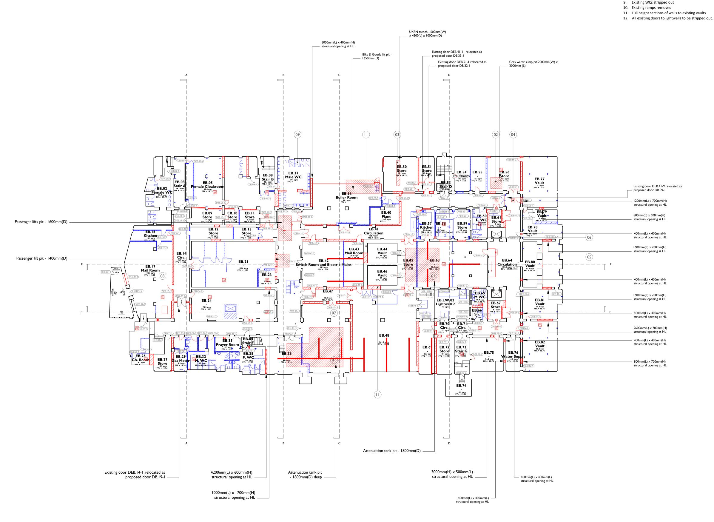
I BASEMENT FLOOR LEVEL PLAN PROPOSED DEMOLITIONS AND STRIP OUT 91000 I:200 @ A I
