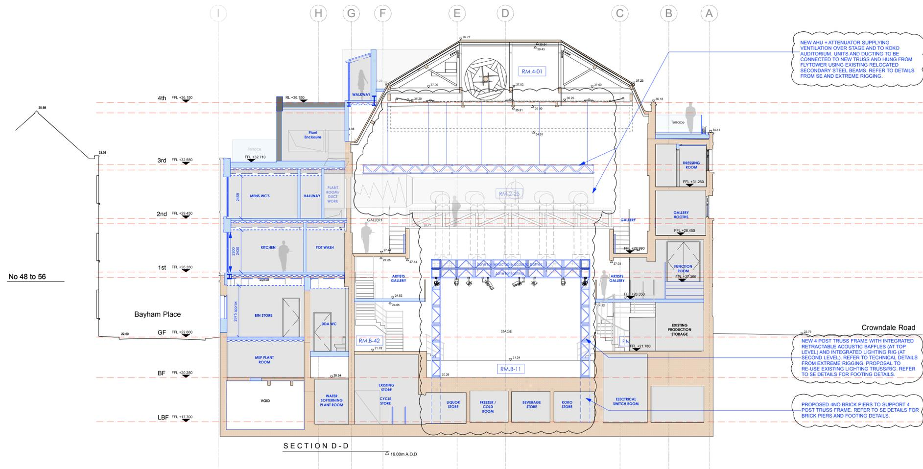
NEW AHU + ATTENUATOR SUPPLYING VENTILATION OVER STAGE AND TO KOKO AUDITORIUM. UNITS AND DUCTING TO BE CONNECTED TO NEW TRUSS AND HUNG FROM FLYTOWER USING EXISTING RELOCATED SECONDARY STEEL BEAMS. REFER TO DETAILS FROM SE AND EXTREME RIGGING.
