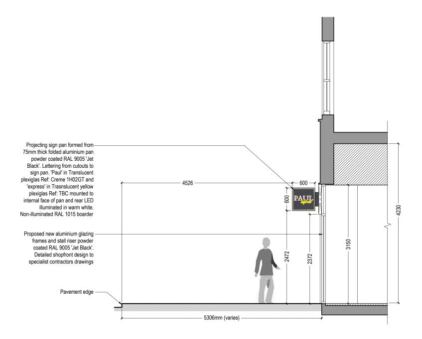
Section A: Typical Section Through Shop Front
