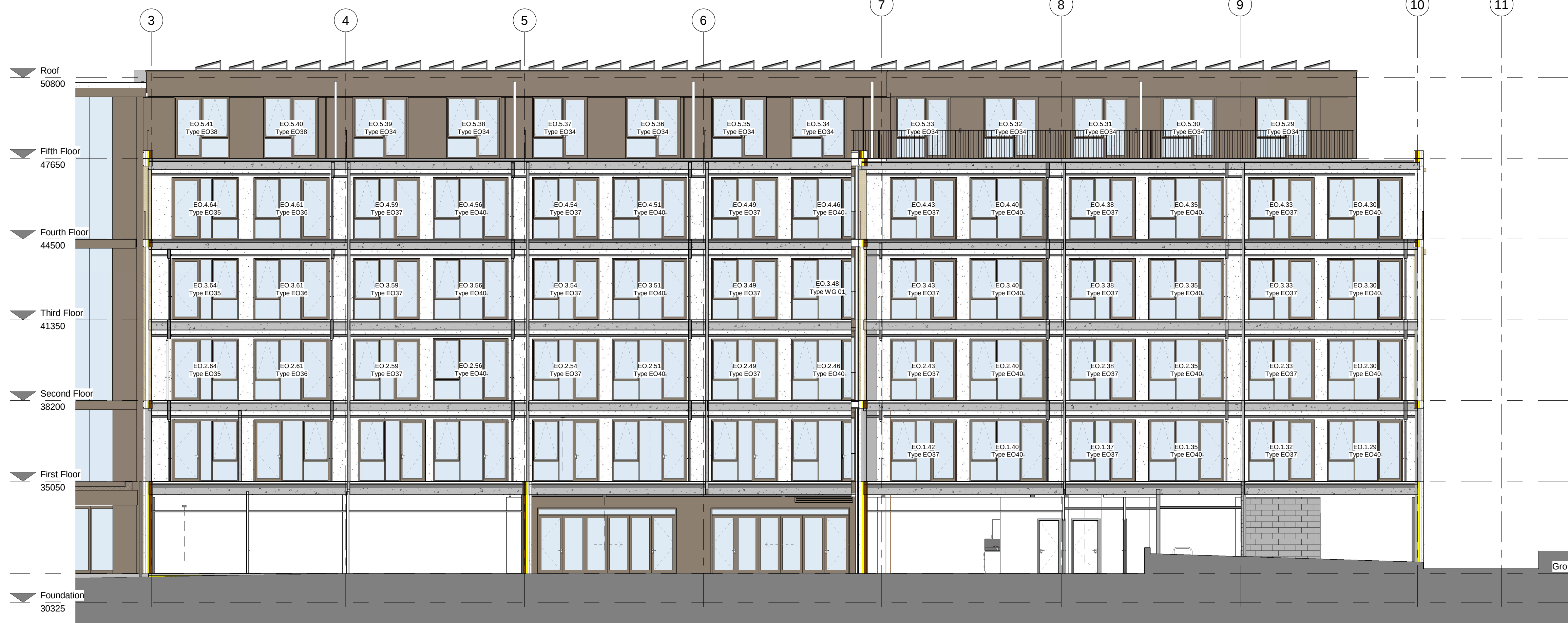
2 | East Elevation taken through Wintergarden 1 : 100
