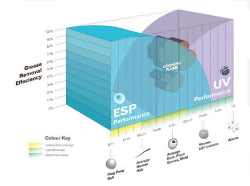
smoke, moisture, gases and particles these vapour: constitute the cooking plume. Typically, they vary in size from 30 microns to sub microns, from combined grease and moisture to vaporised molecules. graph opposite demonstrates effectiveness of the CVL ESP system. Electrostatic precipitation is up to 95% effective at eliminating the particles within the blue shaded area, which includes odours, grease and smoke.
