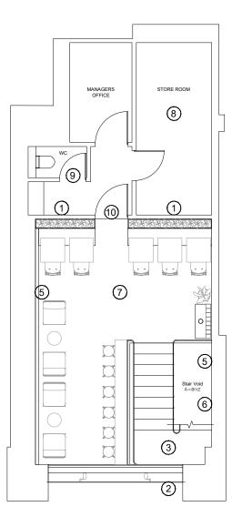
PROPOSED MEZZANINE FLOOR PLAN SCALE 1: 100
