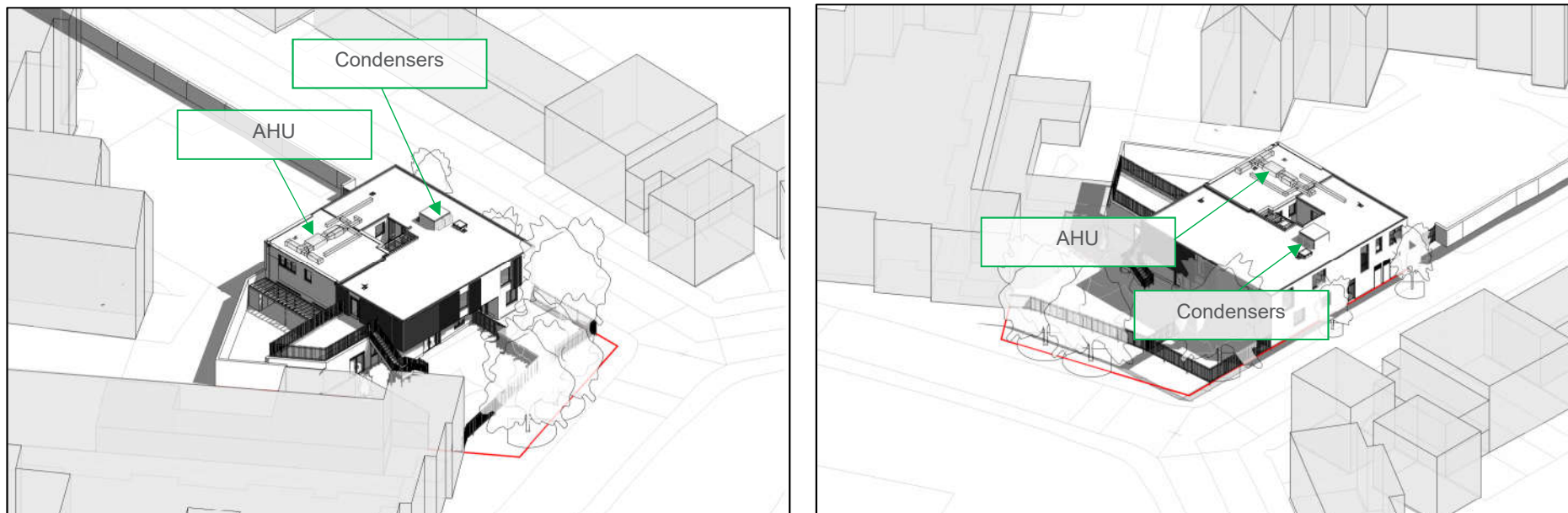
Figure C-2 - Isometric views of the refurbished building showing the proposed condensers and AHU
