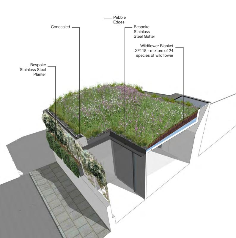
As shown in the section below and the visualization, this multi-layered system will ensure that the 24 species wildflower blanket covers the entirety of the roof, except for a small strip of pebbles against the existing building and the gutter.
