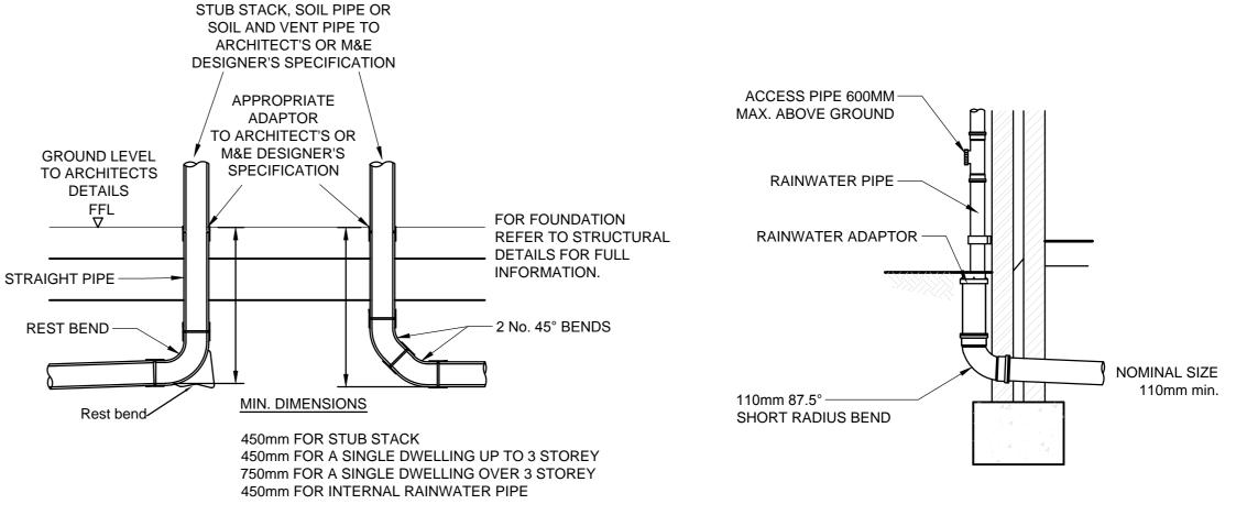
STUB STACK, SOIL VENT PIPE & INTERNAL RAINWATER PIPE DETAIL
