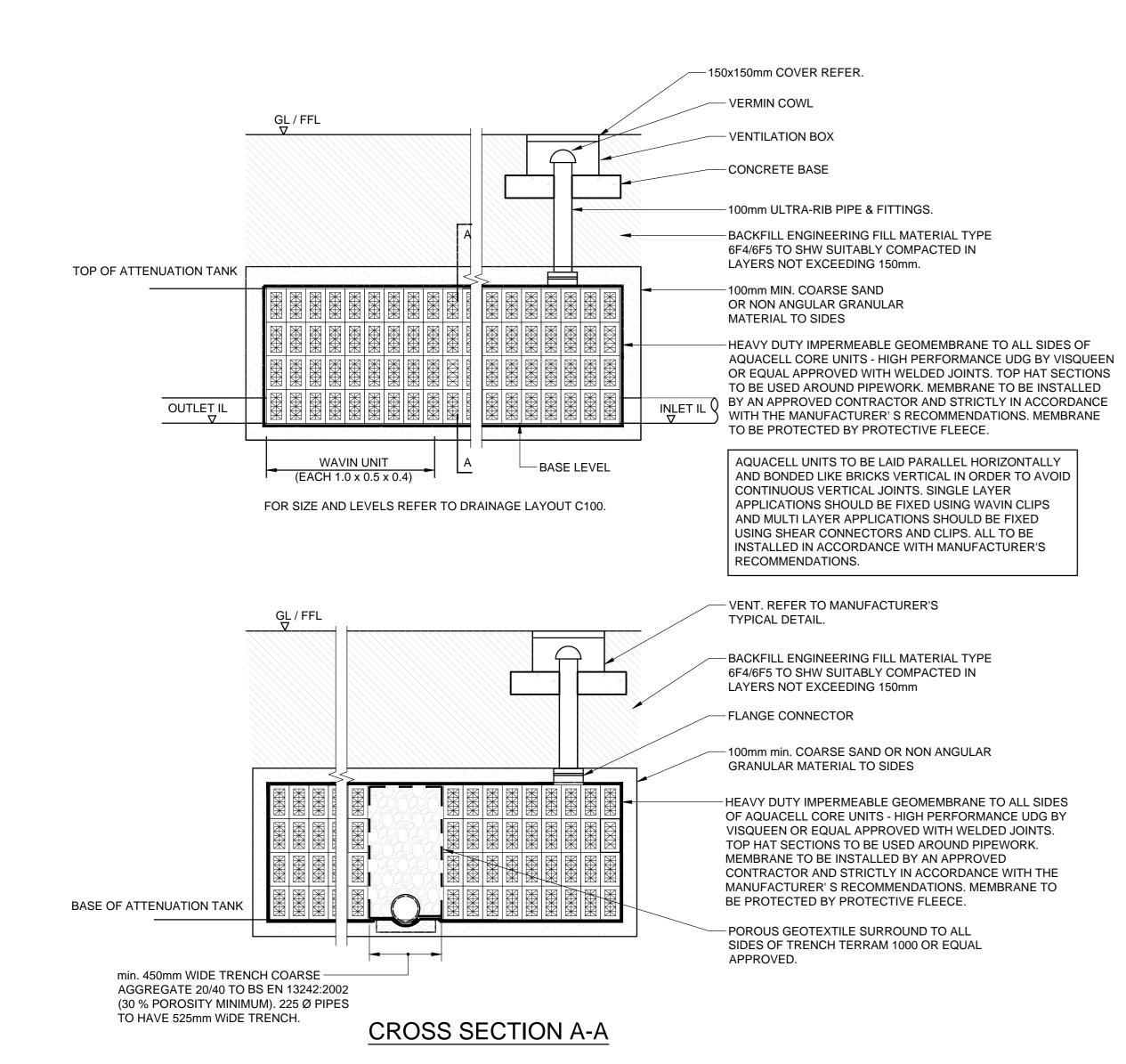
TYPICAL STORM WATER ATTENUATION TANK DETAIL
