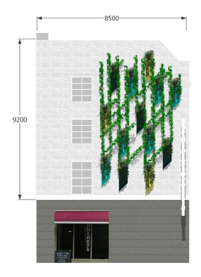
Wire rope: 74 linear meters Vine eyes: 35 Turnbuckles: 15
