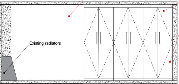
Storewall fixed to a floor and ceiling track for stability- no requirement to fix to walls
