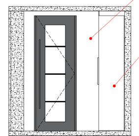
Storewall fixed to a floor and ceiling track for stability- no requirement to fix to walls
