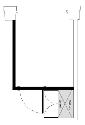
New Partition - see wall details drawing for fixing details
