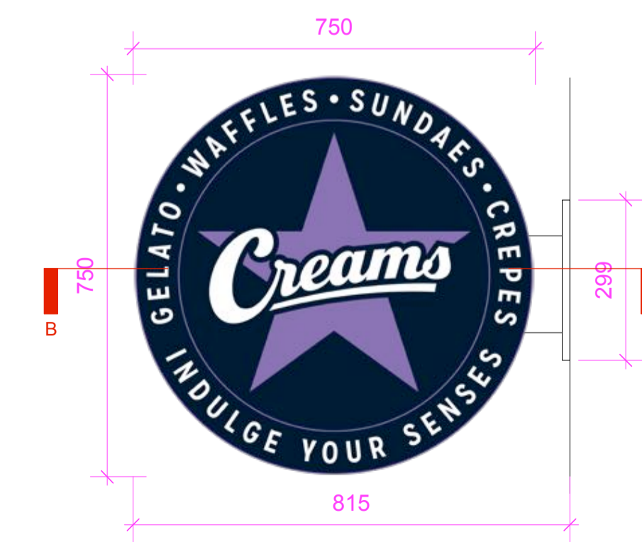
PROJECTING SIGN SIDE VIEW Scale: 1:10
