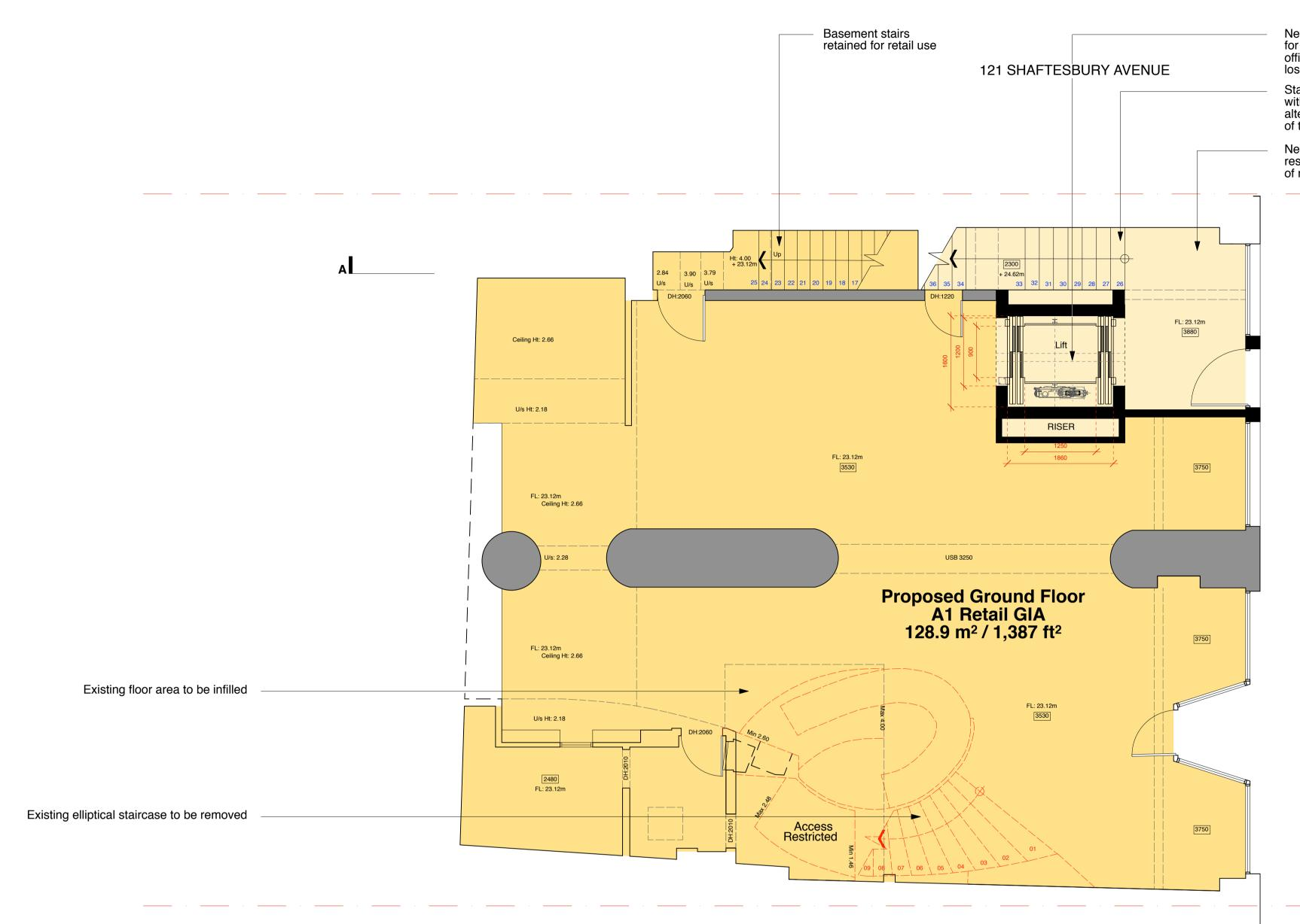
New 6 person through lift shaft, for use by both retail and office, resulting in 2.1m²(22ft²) loss of GIA.
