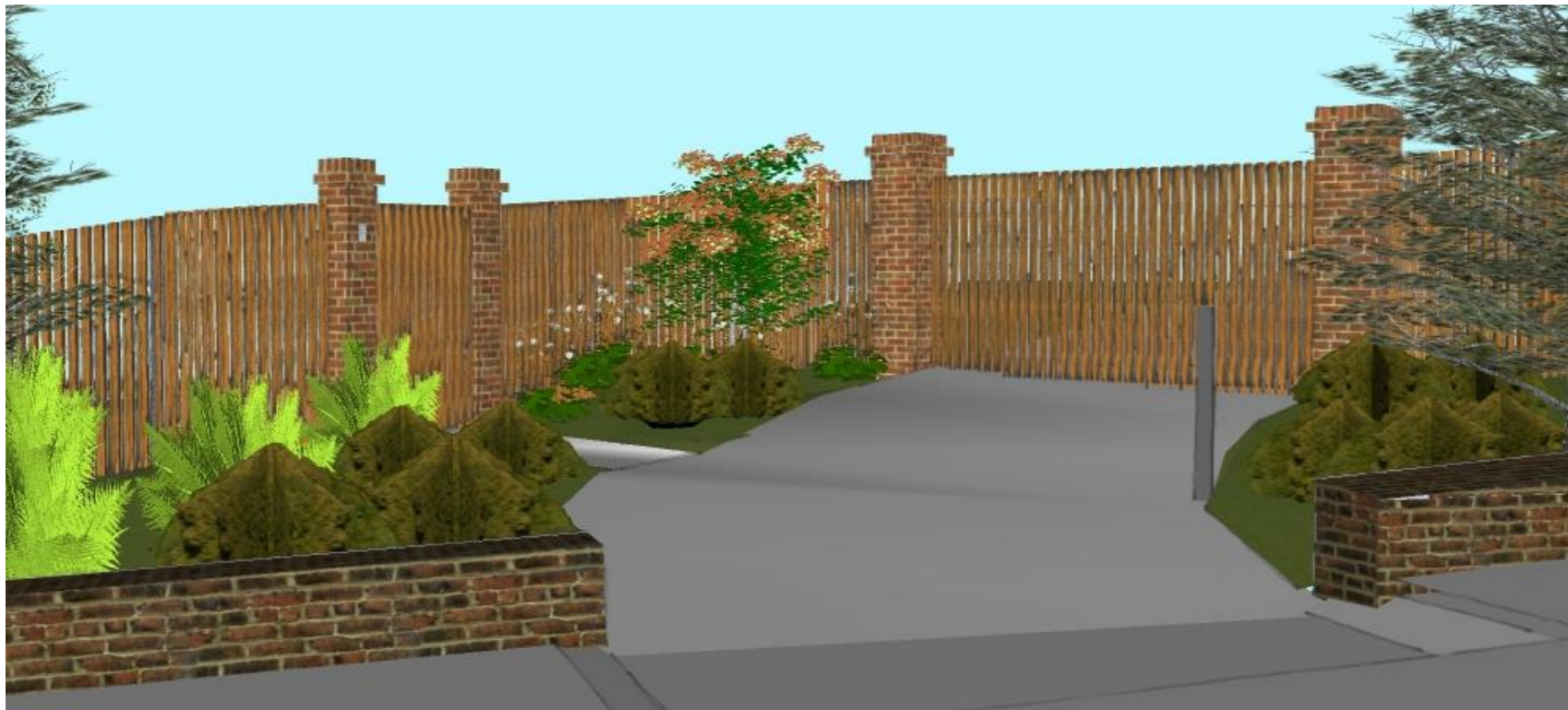
Front boundary fence design showing gate piers (driveway right and pedestrian left)
