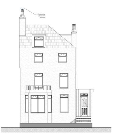
The drawing below shows the rear elevation with the new flue. This new flue will only just be visible to a few top floor flats on Regents Park Road and won't impact the silhouette of the building. These flats will benefit from the removal of the old flue pipes.
