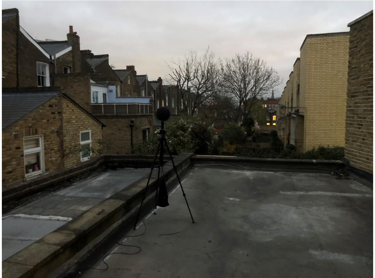
Figure 2: Instrumentation on Roof at First Floor Level
